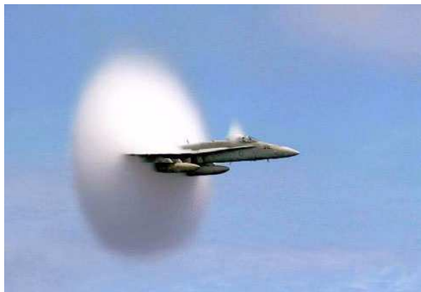
FIG. 2: A photo of the shock wave cone created by the airplane supersonic flight. The cloud is water condensation in the shock wave. (photo taken from http://penguinflight.com/Sonic/ )
